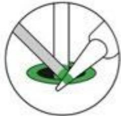
**Do:** While continuing to hold the iron in contact with the leg and metal ring, feed solder into the joint.
