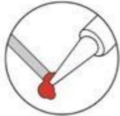
**Don't:** Glob the solder straight onto the iron and try to apply the solder with the iron.
