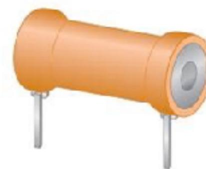
(f) Radial-lead for PC board insertion
