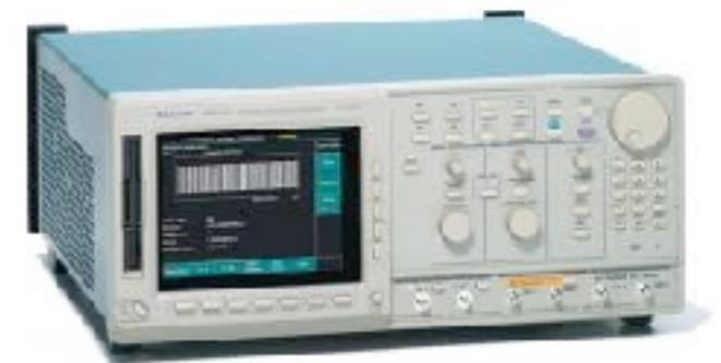
(b) A typical arbitrary waveform generator
