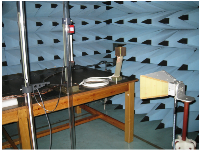
RS for 1 GHz to 2 GHz in vertical position (the following tests used this antenna in the vertical position).
