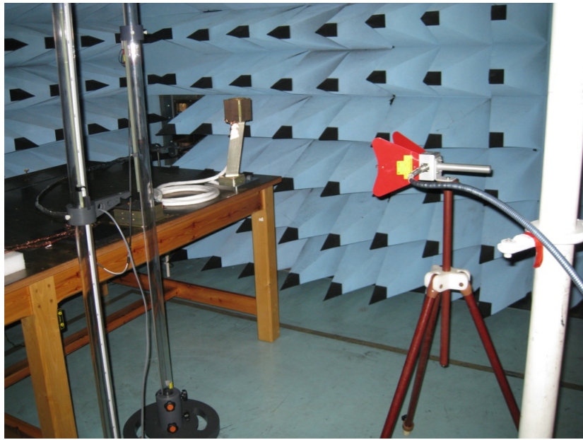
RS for 1 GHz to 2 GHz in horizontal position (the following tests used this antenna in the horizontal position).
